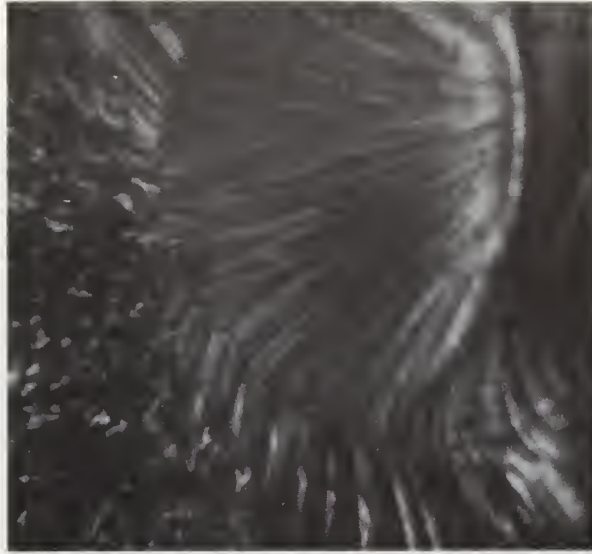
FIGURE 18. OPTICAL MICROGRAPH OF THE FRACTURE SURFACE AT A FLAW OF A TENSILE SPECIMEN; EPON 828 + 5 pph CURING AGENT D. (55X).
